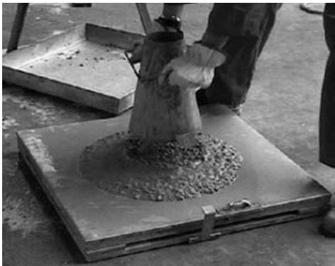
Fig. 1. Slump flow test method
